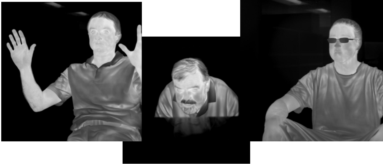
Fig. 10: Longwave infrared images from the 1024x1024 SLS FPA at 77K.
